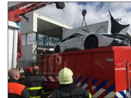
Fully submerging a damaged BMW EV for transport in the Netherlands
